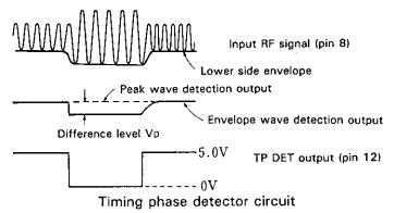
The envelope wave detection circuit detects the lower side envelope of input RF signal. The peak detection circuit detects the level difference VD of the envelope wave detection output. By applying DC to pin 9 the difference detection level (VTH) can be varied. However when pin 9 is open (it is internally biased to 1.3 V), VTH becomes 50 mV, and with a signal where the difference exceeds 50 mV, TP DET output is obtained.
