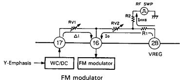
At the figure, (FM modulator) the carrier bias current IO can be adjusted through RV2,. Also, the level (deviation) of signal current Δi can be set with RV1. The HHS current (IHHS) is determined through R1 R2, and RF SWP level.
