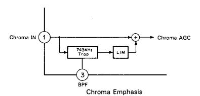
The down converted chroma signal is applied to the chroma Emphasis input, and the amount of emphasis diminishes around fsc (color sub carrier frequency: 743.444 kHz) as it is distanced from fsc, the amount of emphasis grows.
