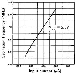
FM MOD Oscillation frequency supply voltage characteristics
