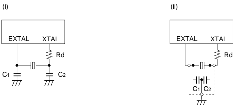
Fig. 8. Recommended oscillation circuit
