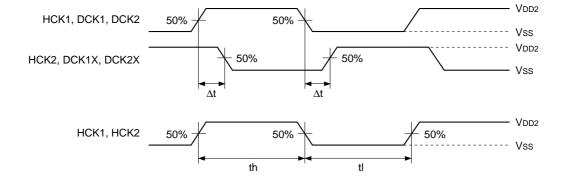
Parallel I/F Block AC Characteristics (Topr = -20 to +75°C, VDD1 =  $2.5 \pm 0.2$ V, VDD2 =  $3.3 \pm 0.3$ V, Vss = 0V)
