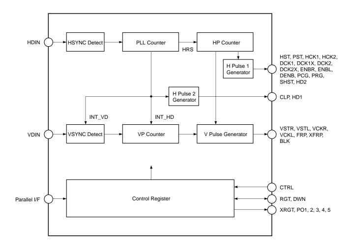
**Timing Generator Block Diagram**
