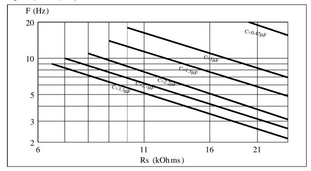
Fig 2.: Spark frequency versus Rs and C
