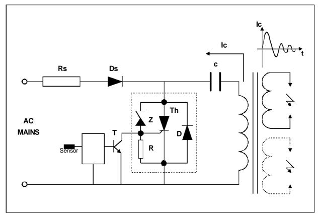
The applications of the FLC02 using the capacitance discharge topology operate in 2 modes :
