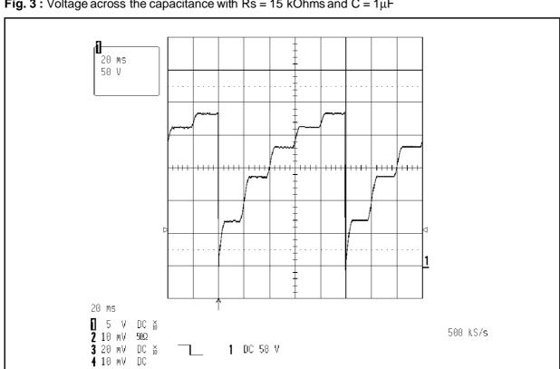
Fig. 3 : Voltage across the capacitance with Rs = 15 kOhms and C =  $1\mu F$
