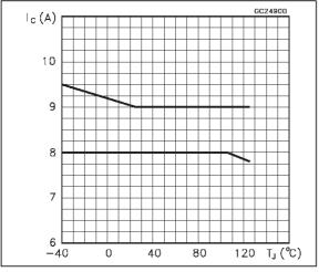
FIGURE 5:  $I_{C(diag2)}$  VS temperature
