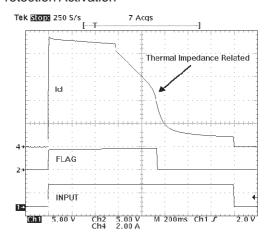
FIG. 4 Single Pulse Typical Es/b Curve
