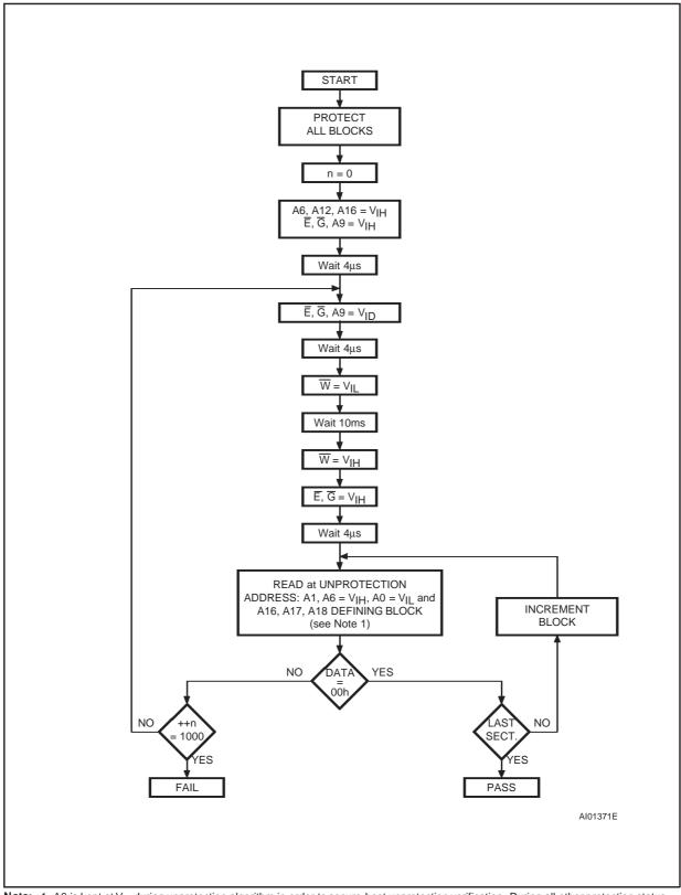
Note: 1. A6 is kept at V<sub>IH</sub> during unprotection algorithm in order to secure best unprotection verification. During all other protection status reads, A6 must be kept at V<sub>IL</sub>.
