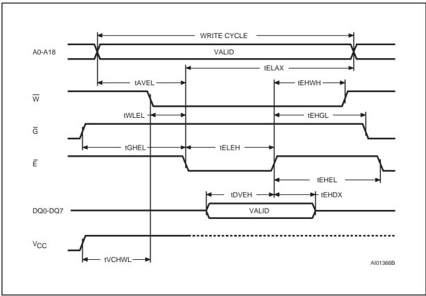
**Note:** Address are latched on the falling edge of  $\overline{E}$ , Data is latched on the rising edge of  $\overline{E}$ .
