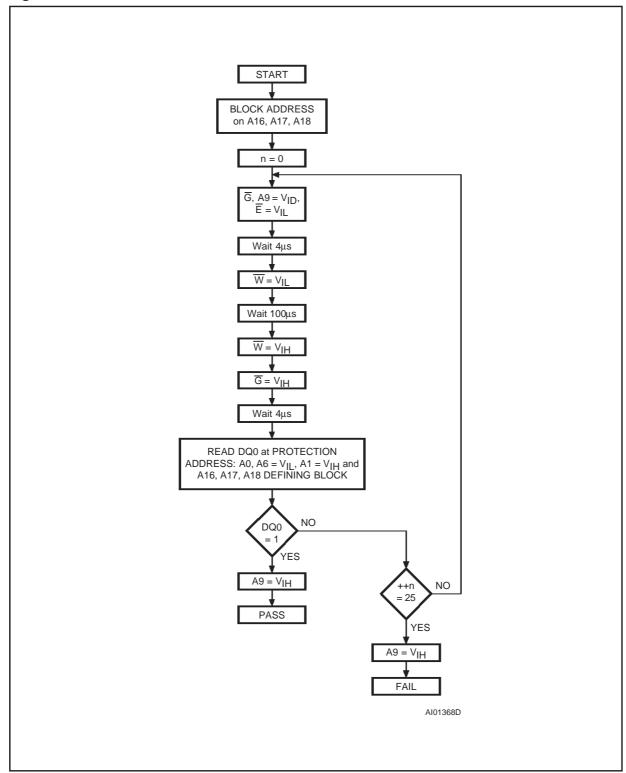
Figure 14. Block Unprotecting Flowchart
