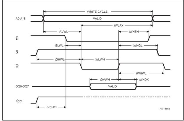
Figure 7. Write AC Waveforms, W Controlled
