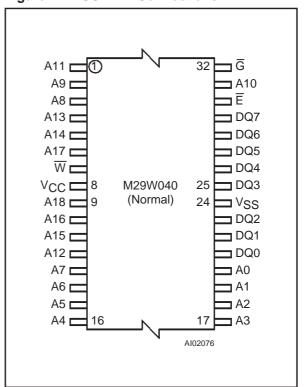
Figure 2C. TSOP Reverse Pin Connections
