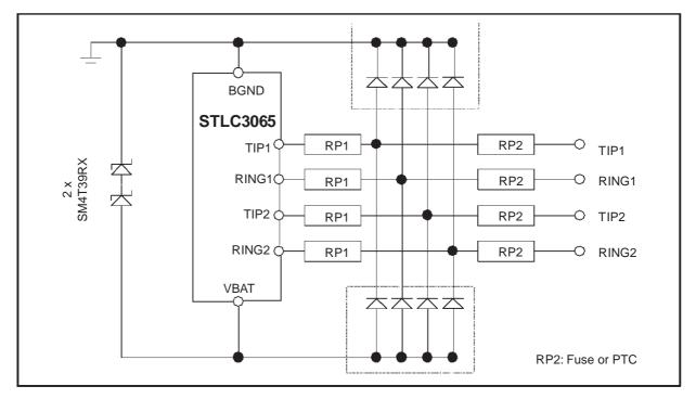
Figure B2. Standard overloltage protection configuration for k20 compliance
