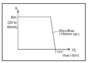
The line status (on/off hook) is monitored by the SLIC core Supervision circuit. The off-hook threshold can be programmed via the external resistor RTH in the range from 5mA to 9mA.
