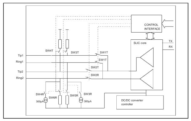
The STLC3065 operating modes will be obtained as combination of the SLIC core status and the dual port configuration.
