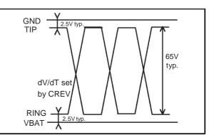
this way a trapezoidal balanced ring waveform (see fig.6).
