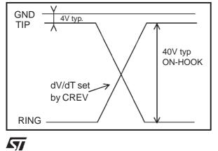
When the control pins set battery reversal the line polarity is reversed with a proper transition time set via an external capacitor (CREV).
