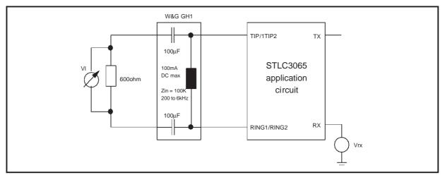
Figure A5. PSRRC Power supply rejection Vpos to 2W port *PSSRC = 20Log/Vn/VI*
