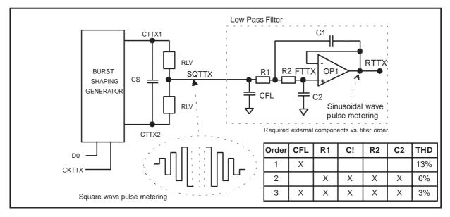
As already mentioned the metering pulse echo cancellation is obtained by means of two external components (RTTX and CTTX) that should match the line impedance at the TTX frequency. This simple network has a double effect:
