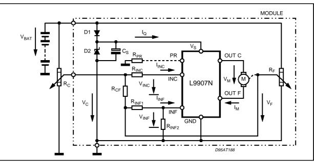
V<sub>C</sub> operating range. For ideal adjusted condition  $V_F = \frac{R_{INF2}}{R_{INF2} + R_{INF2}} \cdot V_C$ :
