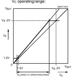
Figure 6: Control to feedback transfer characteristic for proportional regulation with reduced V<sub>C</sub> operating range: rating for  $V_{S}$ . The device features an output disable function in case of control input voltage overdrive.
