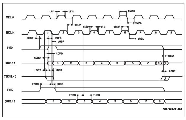
Figure 6: Delayed Data Timing (short frame mode)
