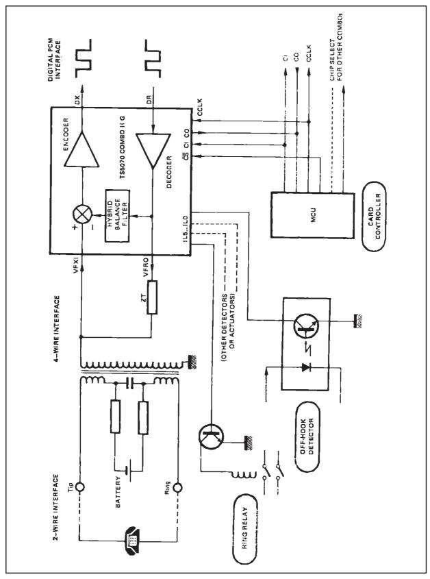
Figure 4: Interface with L3092 + L3000 Silicon SLIC.
