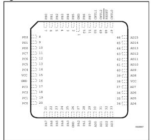
Figure 2B. PQFP Connections
