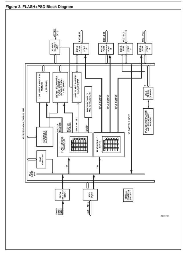
EPROM or Flash memory, or an external programmer. To simplify Flash memory updates, program execution is performed from a secondary Flash memory (for the M89xxF2x) or EEPROM (for the M8913F1x) while the primary Flash memory is being updated. This solution avoids the complicated hardware and software overhead necessary to implement IAP.
