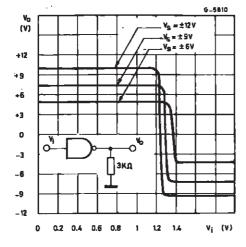
Figure 7 : Transfer Characteristics versus
