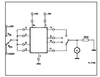
Figure 4 : Output Resistance (power off)
