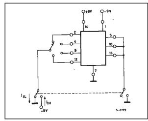
Figure 3 : Output Short-Circuit Current
