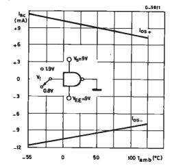
**Figure 10 :** Output Voltage and Current Limiting Characteristics
