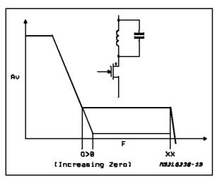
2)The motor capacitance, CM, itself can interfere with the loop, creating double poles. If the gain at higher frequencies is sufficiently high, the double pole slope of 40dB/decade can cause the phase shift to reach 180°, re sulting in oscillation.
