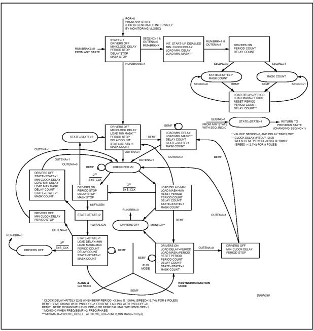
After the next align time-out 192/Falign), the controller enters the Go mode, were the sequencer again double increments the output phase upon detection of the motor's Bemf.
