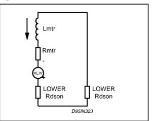
Figure 5-6 is an equivalent circuit of the output stage during the Constant-OFF period. During the OFF time the lower driver for the particular phase beign driven remains ON.
