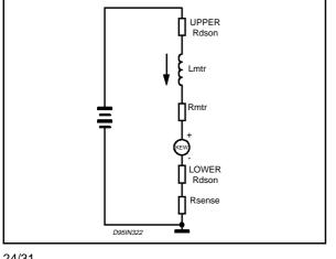
The additional resistance associated with the output stage and sensing resistor are also in series with the motor. If we let Rs equal the total series resistence:
