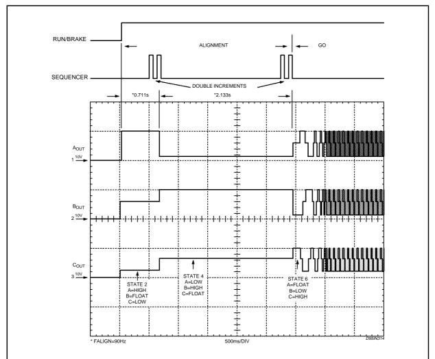
2) **Closed Loop Start-Up** - The Bemf voltage zerocrossings provide timing information so that the motor can be accelerated to steady state speed.
