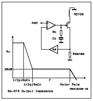
The pole/zero locations are adjusted such that a few dB of gain (typ. 20dB) remains in the transconductance loop at frequencies higher than the zero.
