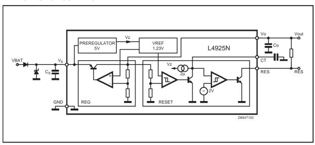
For stability:  $C_S \ge 1\mu F$ ;  $C_O \ge 10\mu F$ ; ESR < 2.5 $\Omega$  at 10 KHz Recommended for application:  $C_S = C_O = 10\mu F$  to  $100\mu F$
