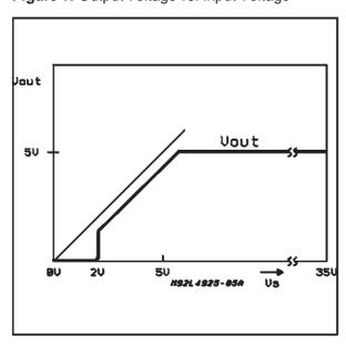
The dropout operation of the standby regulator is maintained down to 3V input supply voltage. The output voltage is regulated up to the transient input supply voltage of 35V. With this feature no functional interruption due to overvoltage pulses is generated.
