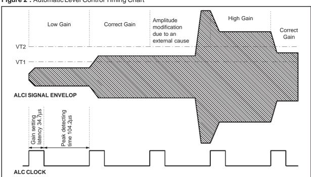
Figure 2: Automatic Level Control Timing Chart
