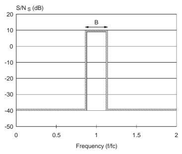
B = 20kHz at 600 Bit/s (BRS = 0) B = 40kHz at 1200 Bit/s -BRS = 1)
