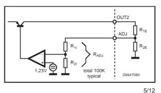
Connecting a resistor divider  $R_{1E}$ ,  $R_{2E}$  to the ADJ, OUT2 pin the output voltage 2 can be programmed to the value of
