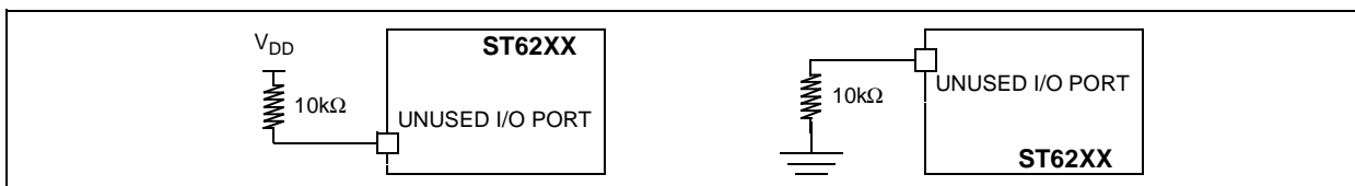
Figure 62. Two typical Applications with unused I/O Pin
