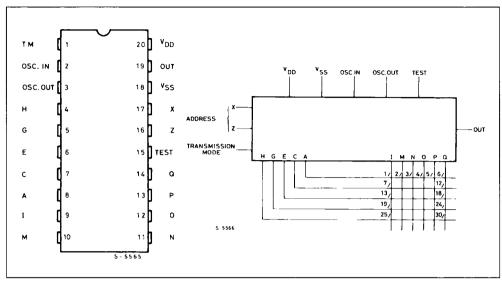
Note: The test pin must be connected to Vss.
