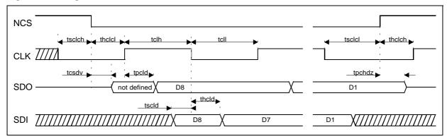
The SPI register data are transferred to the output latch at rising NCS edge. The digital filter between NCS and the output latch ensures that the data are transferred only after 8 CLK cycles or multiple of 8 CLK cycles since the last NCS falling edge. The NCS changes only at low CLK.
