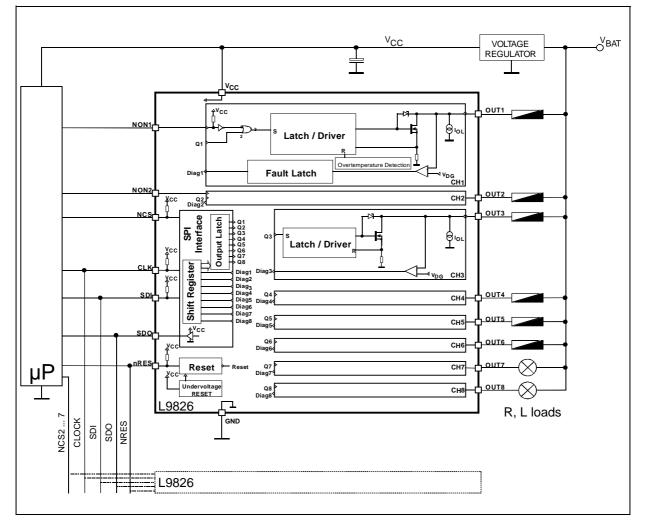
For higher current driving capability two outputs of the same kind can be paralleled. In this case the maximum flyback energy should not exceed the limit value for single output.
