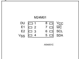
Note: 1. DU = Don't Use (should be left unconnected, or tied to  $V_{SS}$ )
