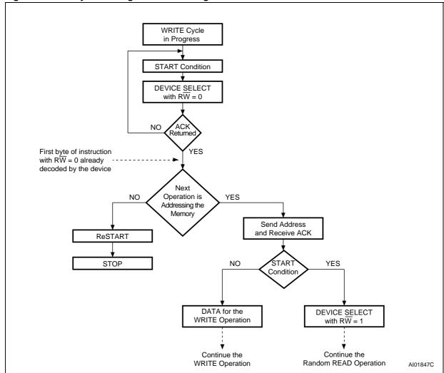
Figure 8. Write Cycle Polling Flowchart using ACK
