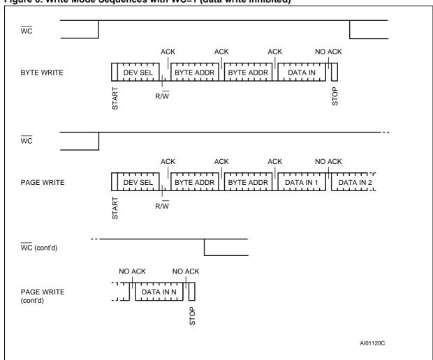
Figure 6. Write Mode Sequences with WC=1 (data write inhibited)
