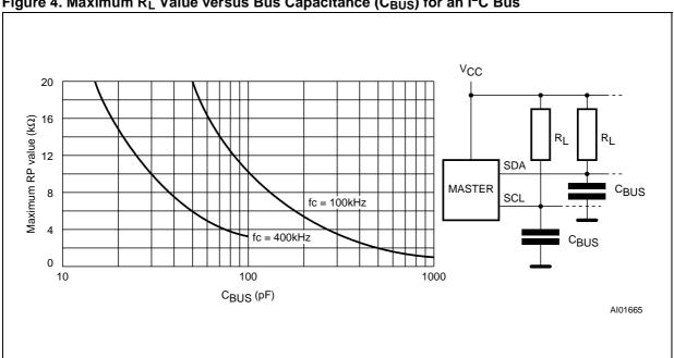
Figure 4. Maximum R<sub>L</sub> Value versus Bus Capacitance (C<sub>BUS</sub>) for an I<sup>2</sup>C Bus
