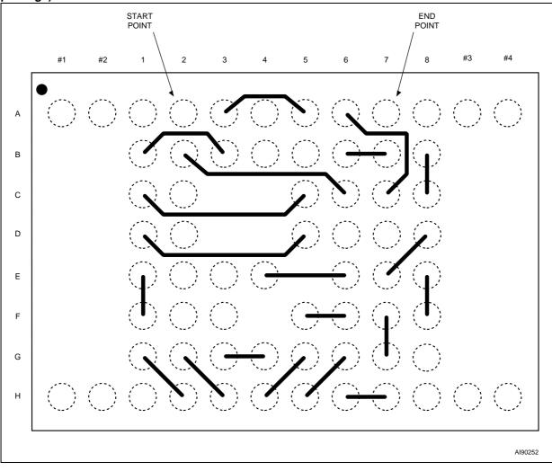
Figure 27. Stacked LFBGA66 Daisy Chain - PCB Connections proposal (Top view through package)
