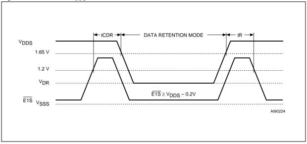
Figure 24. SRAM Low V<sub>DDS</sub> Data Retention AC Waveforms, E2S Controlled
