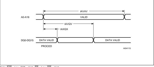
Note:  $\overline{E1S}$  = Low, E2S = High,  $\overline{GS}$  = Low,  $\overline{WS}$  = High.
