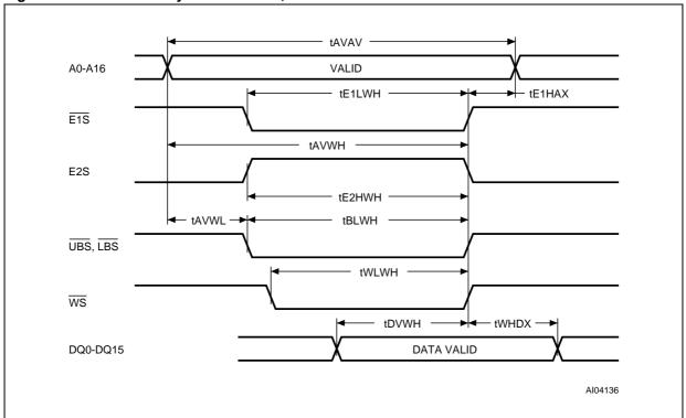
Figure 21. SRAM Write Cycle Waveform, UBS and LBS Controlled
