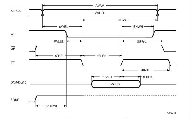
Note: Address are latched on the falling edge of  $\overline{EF}$ , Data is latched on the rising edge of  $\overline{EF}$ .
