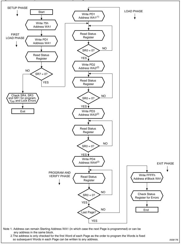
Figure 37. Quadruple Enhanced Factory Program Flowchart
