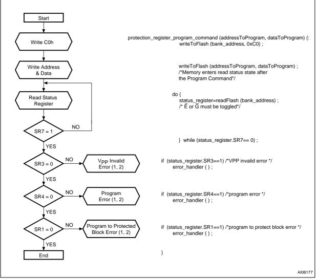
Figure 35. Protection Register Program Flowchart and Pseudo Code
