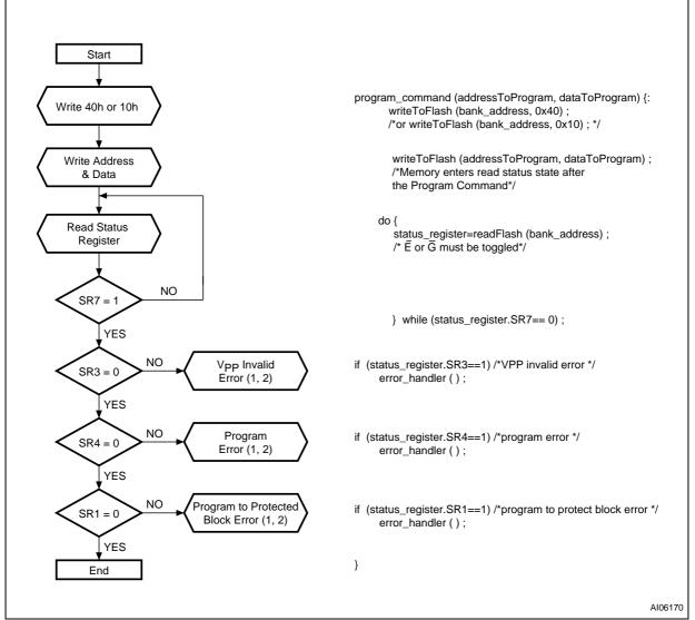
Note: 1. Status check of SR1 (Protected Block), SR3 (V<sub>PP</sub> (V<sub>PPF</sub>) Invalid) and SR4 (Program Error) can be made after each program operation or after a sequence.
