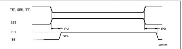
Figure 21. SRAM Chip Enable or UBS/LBS Controlled, Standby AC Waveforms
