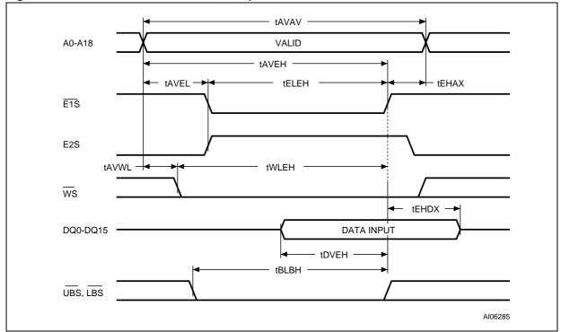
Figure 23. SRAM Write AC Waveforms, Chip Enable Controlled
