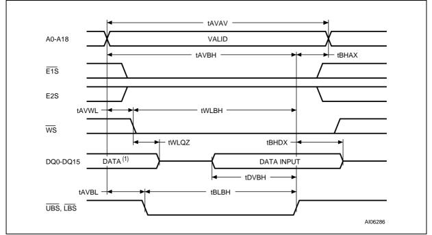
Note: 1. During this period DQ0-DQ15 are in output state and input signals should not be applied.
