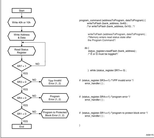
Note: 1. Status check of SR1 (Protected Block), SR3 (VPP Invalid) and SR4 (Program Error) can be made after each program operation or after a sequence.
