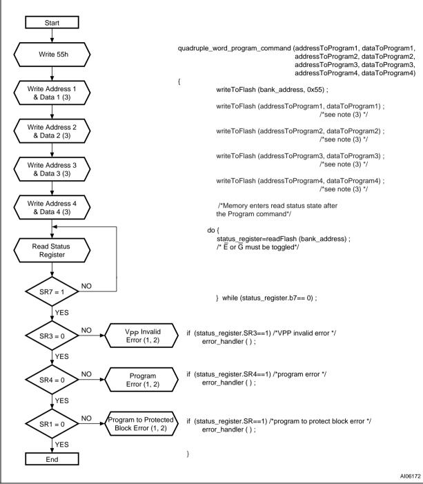
Note: 1. Status check of SR1 (Protected Block), SR3 (VPP Invalid) and SR4 (Program Error) can be made after each program operation or after a sequence.
