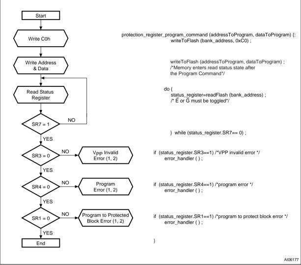
Note: 1. Status check of SR1 (Protected Block), SR3 (V<sub>PP</sub> Invalid) and SR4 (Program Error) can be made after each program operation or after a sequence.
