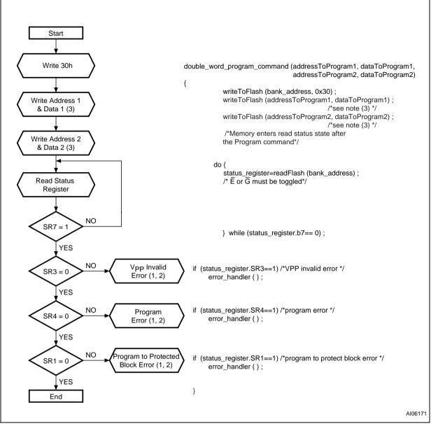
Note: 1. Status check of b1 (Protected Block), b3 (V<sub>PP</sub> Invalid) and b4 (Program Error) can be made after each program operation or after a sequence.
