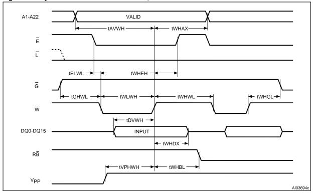
Figure 15. Asynchronous Write AC Waveform, Write Enable Controlled
