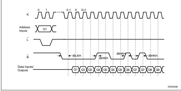
Note: In this example the Burst Configuration Register is set with M2-M0 = 001 (Burst Length = 4 Words or Double Words), M6 = 1 (Valid Clock Edge = Rising Clock Edge), M7 = 0 or 1 (Burst Type = Interleaved or Sequential), M9 = 0 (Y-Latency = 1), M14-M11 = 0011 (X-Latency = 8) and M15 = 0 (Read Select = Synchronous Burst Read), other bits are don't care.
