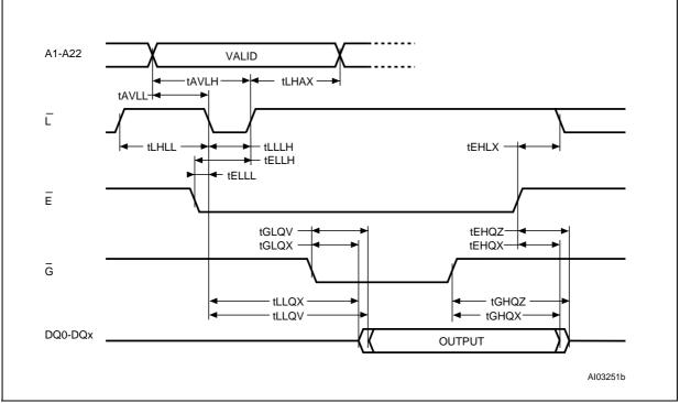
Figure 13. Asynchronous Latch Controlled Bus Read AC Waveforms
