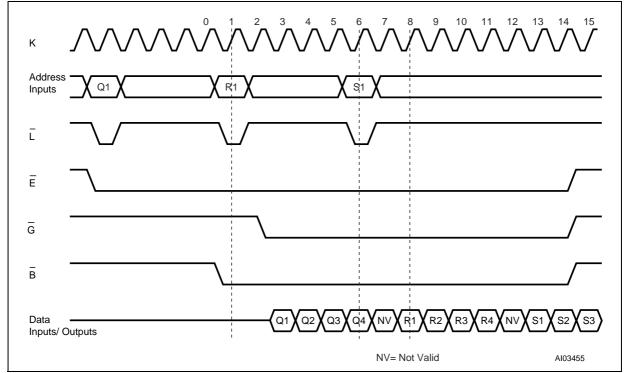
Figure 8. Example Synchronous Pipelined Burst Read Operation
