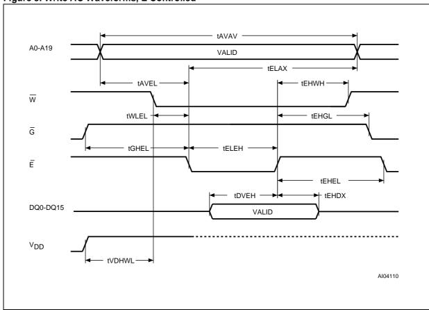
Figure 8. Write AC Waveforms,  $\overline{\mathbf{E}}$  Controlled
