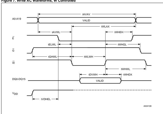
Figure 7. Write AC Waveforms,  $\overline{\mathbf{W}}$  Controlled
