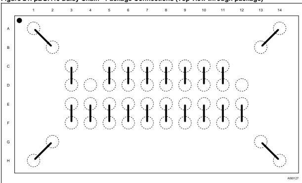
Figure 21. µBGA46 Daisy Chain - Package Connections (Top view through package)
