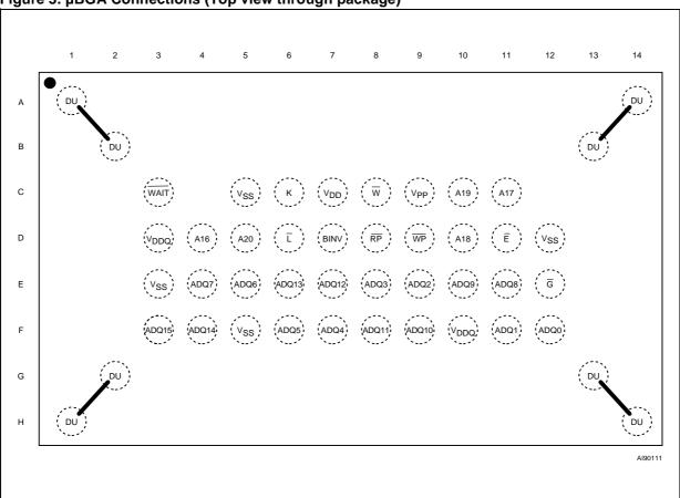
Figure 3. µBGA Connections (Top view through package)
