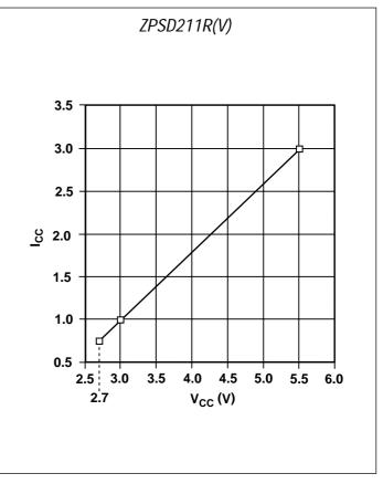
Figure 17. Normalized  $I_{CC}$  (AC) ( $V_{CC} = 3.0 \text{ V}$ )
