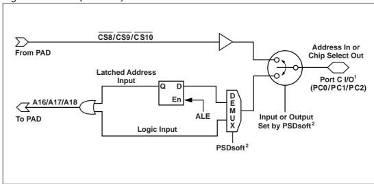
NOTES: 1. Port C pins can be individually configured as inputs or outputs, but not both.
