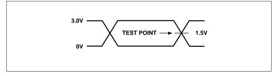
Figure 22B. AC Testing Input/Output Waveform (3 V Versions)
