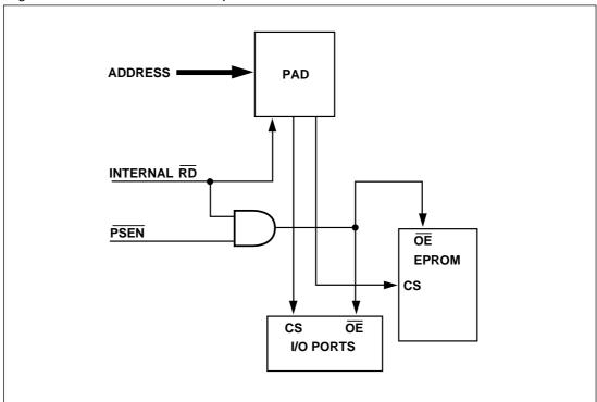
Figure 10. 8031-Compatible Separate Code and Data Address Spaces
