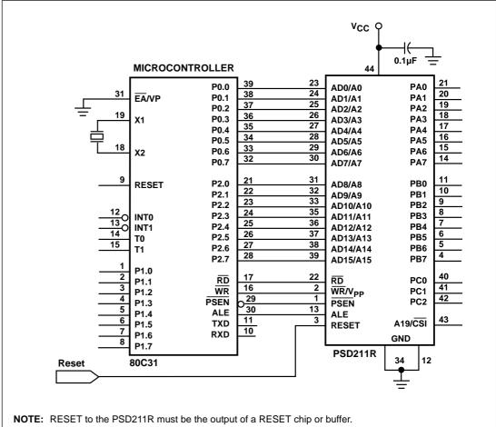
OTE: RESET to the PSD211R must be the output of a RESET chip or buffer.
