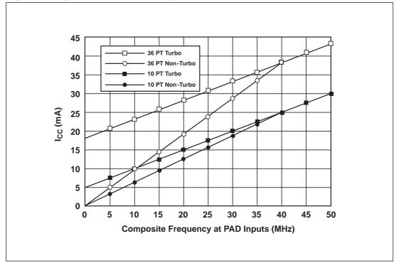
Figure 14. Typical  $I_{CC}$  vs. Frequency for the PAD ( $V_{CC} = 3 V$ )
