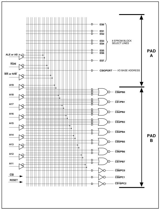
**NOTES:** 1.  $\overline{CSI}$  is a power-down signal. When high, the PAD is in stand-by mode and all its outputs become non-active. See Tables 7A and 7B.
