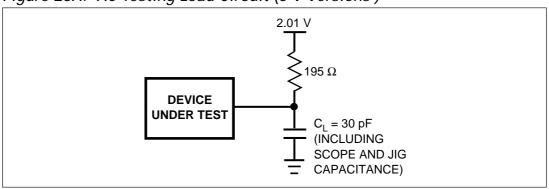
Figure 23B. AC Testing Load Circuit (3 V Versions)
