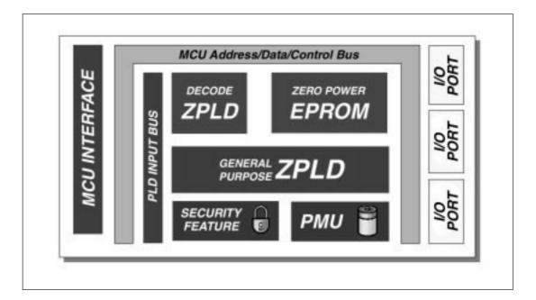
The PSD211R family architecture (Figure 1) can efficiently interface with, and enhance, almost any 8-bit multiplexed microcontroller system. This solution provides microcontrollers the following:
