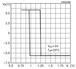
**Figure 2 :** Driver Voltage Transfer Characteristics for Receiver Inputs
