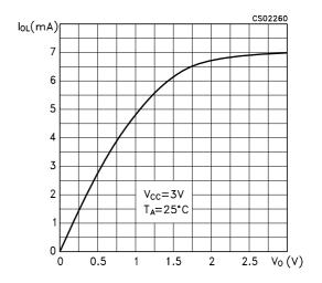
Figure 4 : Output Current vs Output High Voltage
