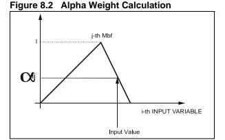
After loading the input values by using the LDFR assembler instruction, the user can start the fuzzy inference by using the FUZZY assembler instruction. During fuzzyfication: input data is transformed in the activation level (alpha weight) of the Mbf's.
