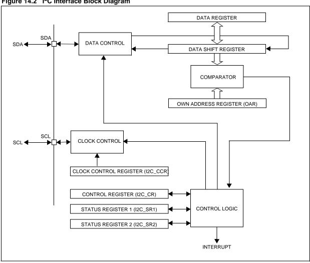
Figure 14.2 I<sup>2</sup>C Interface Block Diagram
