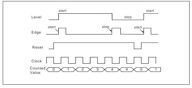
TxSTRT signal starts/stops the Timer from counting only if the peripherals are configured in Timer mode. The Timers are started by writing 1 in the TXSTRT bit of the PWMx\_CR1 and are stopped by writing 0. This signal can be generated internally and/or externally by forcing the TSTRT pin (only TIMER0).
