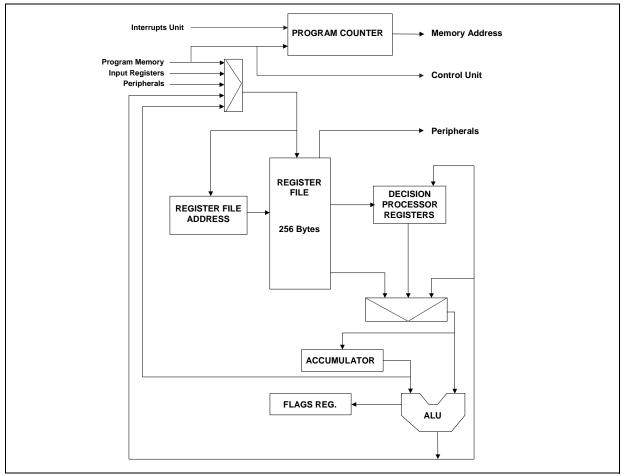
The DPU receives, stores and sends the instructions deriving from the Program/Data Memory, Register File or from the peripherals. It is controlled by the CU on the basis of the decoded instruction. The Fuzzy registers store the partial results of the fuzzy computation. The accumulator register is used by the ALU and is not accessible directly: the instructions used by the ALU can address all the Register File locations as operands, allowing a more compact code and a faster execution.
