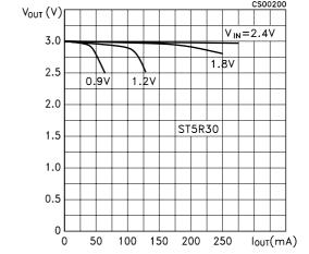
Figure 2: Output Voltage vs Output Current
