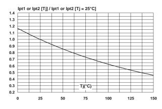
**Fig. 3:** Relative variation of direct pilot voltage versus junction temperature (typical values).
