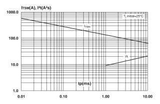
Fig. 1-2: Non repetitive surge peak on-state current (sinusoidal pulse) and corresponding value of 12+
