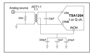
Figure 4 represents the biasing of a differential input signal in AC-coupled differential input configuration. Both inputs VIN and VINB are centered around the common mode voltage, that can be let internal or fixed externally.
