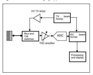
The transducer is a piezoelectric ceramic such as zirconium titanate. The whole array can reach up to 512 channels.
