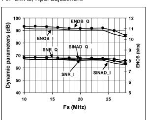
**Distortion vs. Fs** Fin=5MHz; Rpol adjustment
