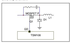
The RC components should realize a time constant corresponding to one tenth of the switching time constant of the TSM108 (i.e. in our example, the oscillator frequency is set to  $10\mu s$  corresponding to 100kHz, therefore, the RC couple should realise a time constant close to  $1\mu s$ ).
