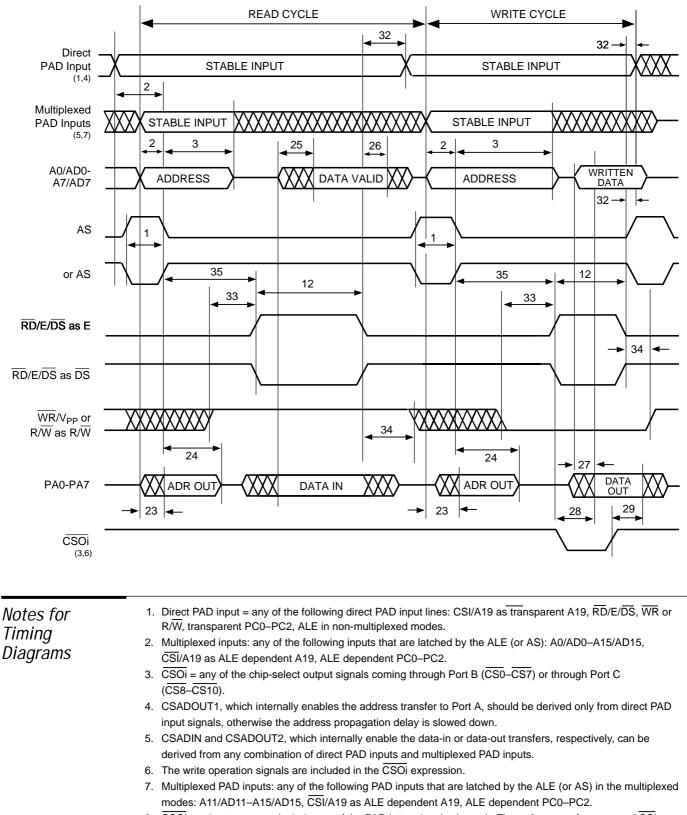
Figure 40. Port A as ADO–AD7 Timing (Track Mode) Using  $R/\overline{W}$ , E or  $R/\overline{W}$ ,  $\overline{DS}$  (PSD3X2/3X3)
