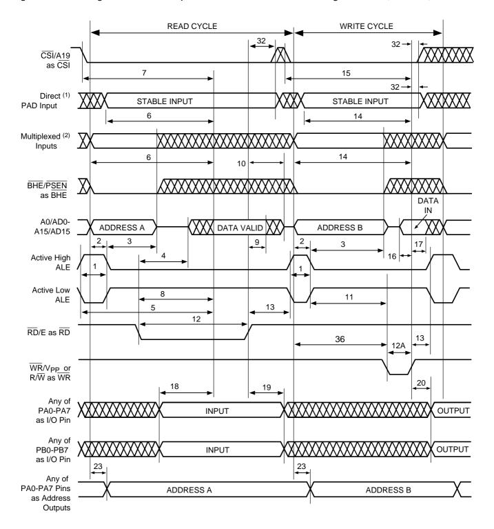
Figure 24. Timing of 16-Bit Multiplexed Address/Data Bus Using RD, WR (PSD3X1)
