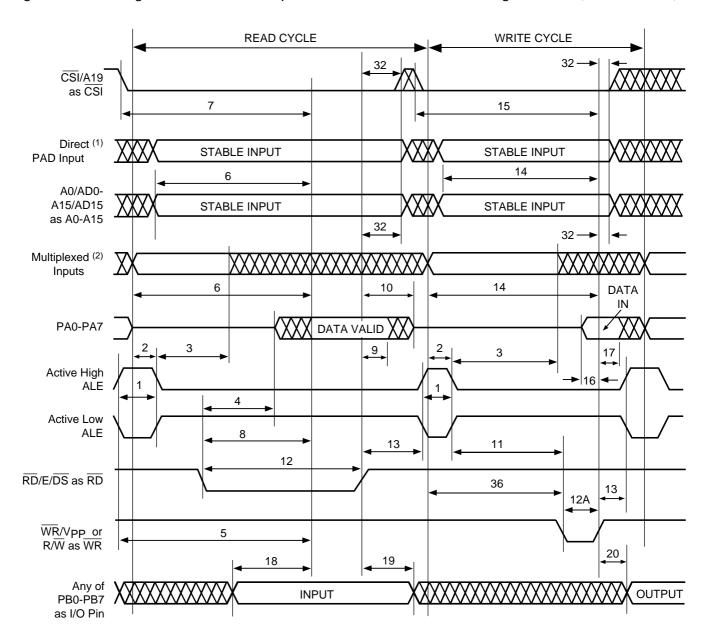
Figure 29. Timing of 8-Bit Non-Multiplexed Address/Data Bus Using RD, WR (PSD3X2/3X3)
