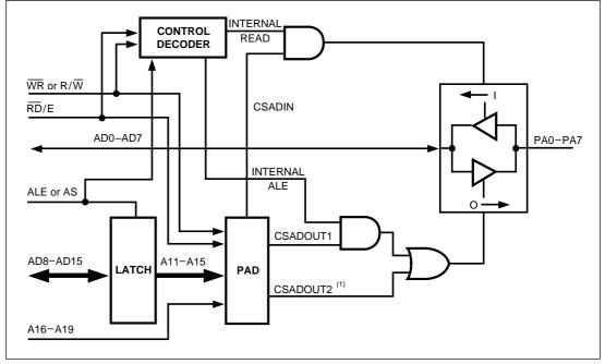
**NOTE:** 1. The expression for CSADOUT2 must include the following write operation cycle signals: For CRRWR = 0, CSADOUT2 must include  $\overline{WR} = 0$ . For CRRWR = 1, CSADOUT2 must include E = 1 and R/W = 0.
