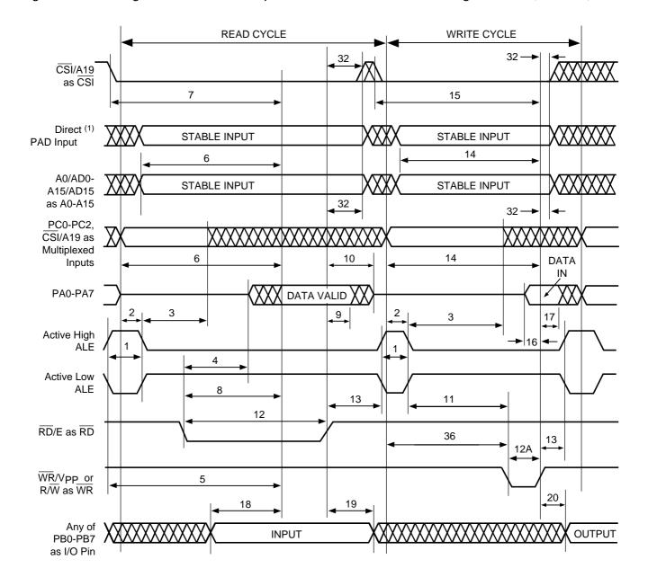
Figure 28. Timing of 8-Bit Non-Multiplexed Address/Data Bus Using RD, WR (PSD3X1)
