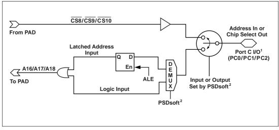
**NOTES:** 1. Port C pins can be individually configured as inputs **or** outputs, but **not** both. Pins can be individually configured as address or logic and latched or transparent, except for the 3X1 devices, which must be set to all address or all logic.
