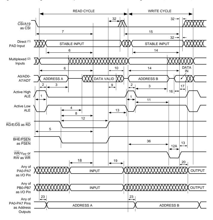
Figure 21. Timing of 8-Bit Multiplexed Address/Data Bus Using RD, WR (PSD3X2/3X3)
