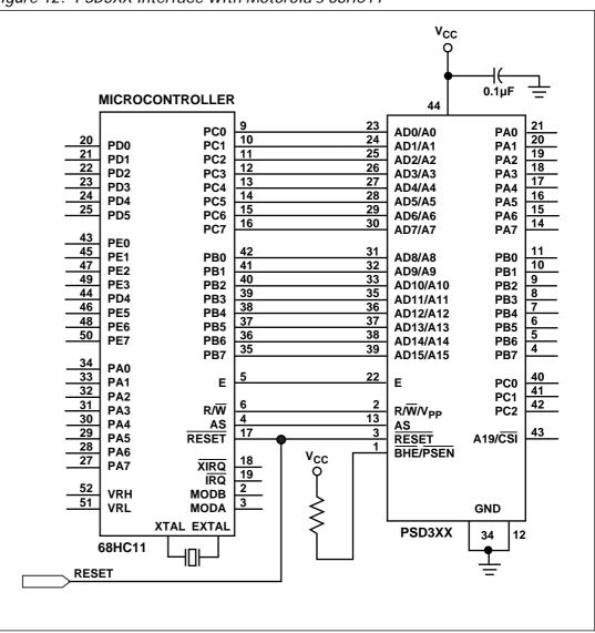
Figure 12. PSD3XX Interface With Motorola's 68HC11
