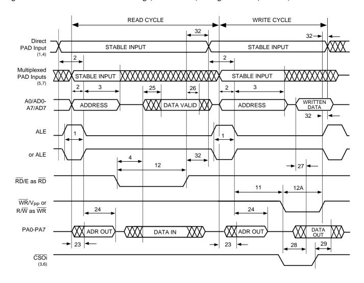
Figure 37. Port A as ADO–AD7 Timing (Track Mode) Using RD, WR (PSD3X1)
