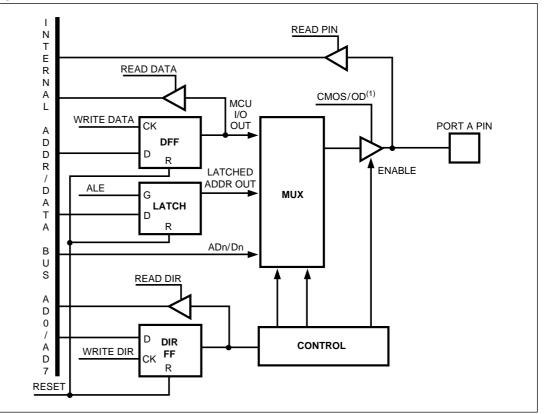
NOTE: 1. CMOS/OD determines whether the output is open drain or CMOS.
