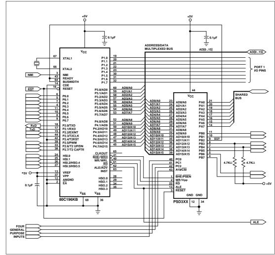
Figure 13. PSD3XX Interface With Intel's 80C196KB
