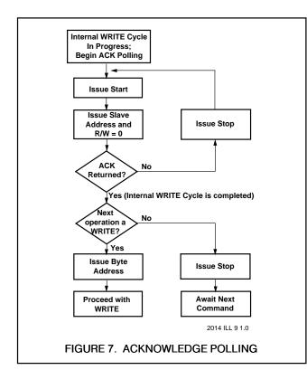
To poll the device, give it a START condition, followed by a slave address for a WRITE operation (See Figure 7).
