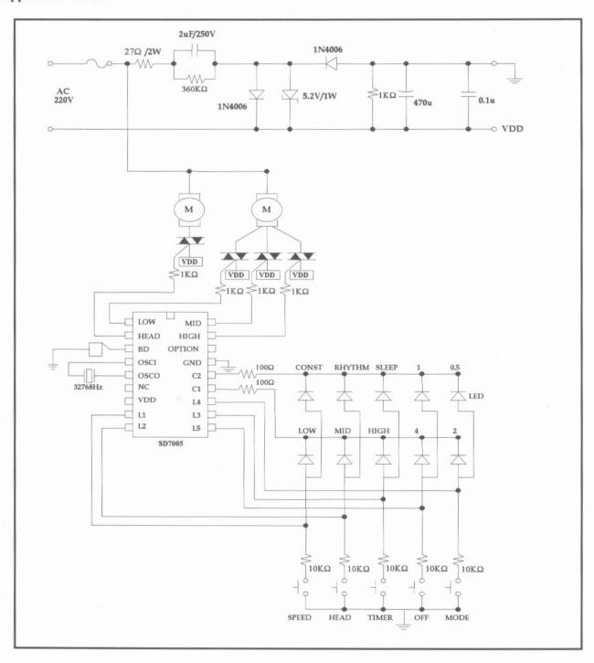
Fig 1. SD7005 Typical Application Circuit.
