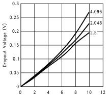
Dropout Voltage vs Load Current
