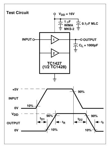
Figure 2. Non-Inverting Driver Switching Time
