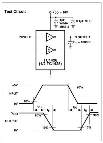
Figure 1. Inverting Driver Switching Time
