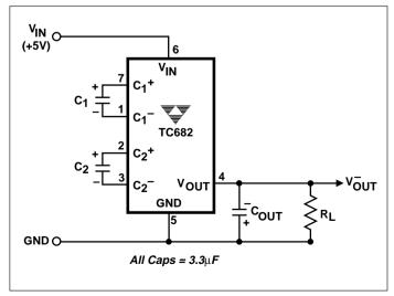
Figure 1. TC682 Test Circuit
