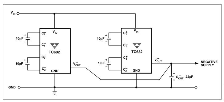
Figure 5. Paralleling TC682 for Lower Output Source Resistance
