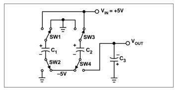
Figure 2. Charge Pump - Phase 1
