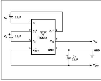
Figure 4. Inverting Voltage Doubler
