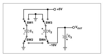
Figure 3. Charge Pump - Phase 2
