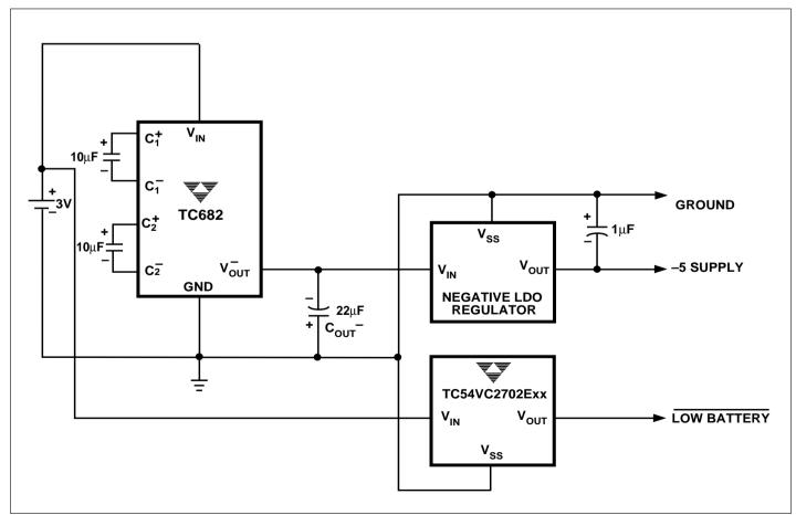
Figure 6. Negative Supply Derived from 3V Battery
