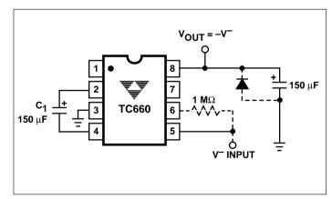
Figure 11. Positive Voltage Multiplier
