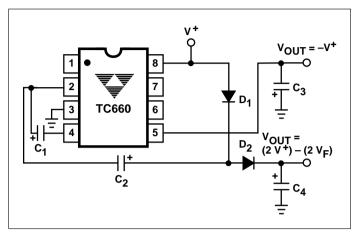
Figure 10. Combined Negative Converter and Positive Multiplier
