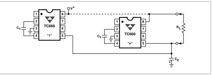
Figure 4. Paralleling Devices Lowers Output Impedance
