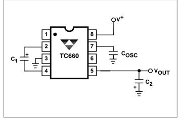
Figure 7. Lowering Oscillator Frequency
