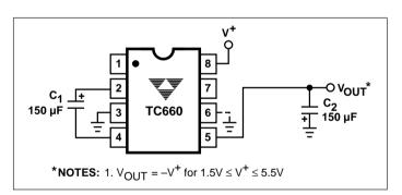
Figure 3. Simple Negative Converter
