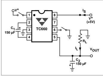
Figure 1. TC660 Test Circuit (Inverter)
