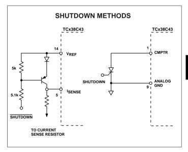
Shutdown can be accomplished by either pulling  $I_{SENSE}$  above 1 volt or pulling CMPTR, pin 1 to GND. This will set the PWM latch so that the output will remain low until the next clock pulse after the shutdown condition is removed.
