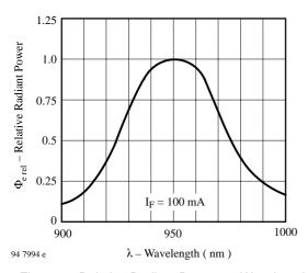
Figure 9. Relative Radiant Power vs. Wavelength
