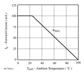
Figure 2. Forward Current vs. Ambient Temperature
