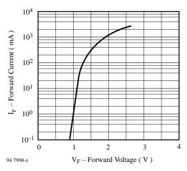
Figure 4. Forward Current vs. Forward Voltage
