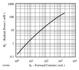
Figure 7. Radiant Power vs. Forward Current
