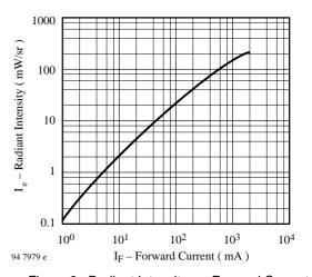
Figure 6. Radiant Intensity vs. Forward Current
