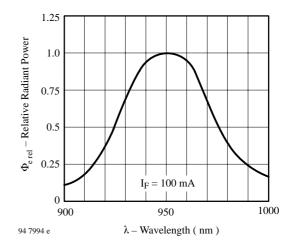
Figure 8. Relative Radiant Power vs. Wavelength
