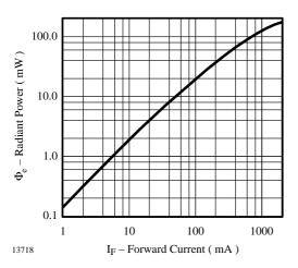
Figure 6. Radiant Power vs. Forward Current
