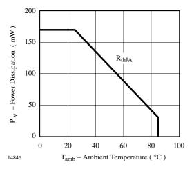
Figure 1. Power Dissipation vs. Ambient Temperature
