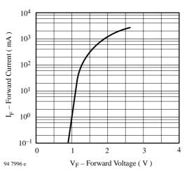
Figure 3. Forward Current vs. Forward Voltage
