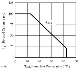
Figure 2. Forward Current vs. Ambient Temperature
