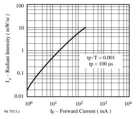
Figure 5. Radiant Intensity vs. Forward Current
