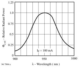
Figure 9. Relative Radiant Power vs. Wavelength
