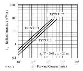
Figure 6. Radiant Intensity vs. Forward Current
