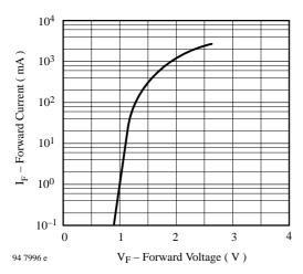
Figure 4. Forward Current vs. Forward Voltage
