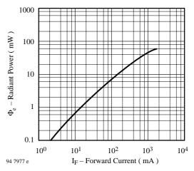
Figure 7. Radiant Power vs. Forward Current
