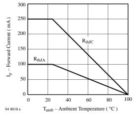
Figure 2. Forward Current vs. Ambient Temperature
