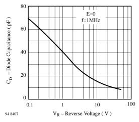
Figure 5. Diode Capacitance vs. Reverse Voltage
