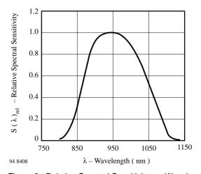
Figure 6. Relative Spectral Sensitivity vs. Wavelength
