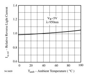
Figure 2. Relative Reverse Light Current vs.
