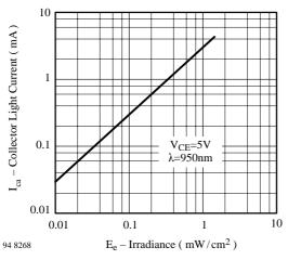
Figure 4. Collector Light Current vs. Irradiance
