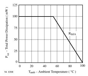
Figure 1. Total Power Dissipation vs.
