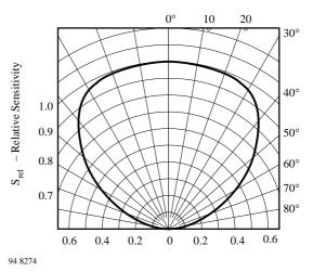
Figure 10. Relative Radiant Sensitivity vs. Angular Displacement
