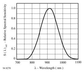
Figure 8. Relative Spectral Sensitivity vs. Wavelength
