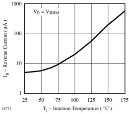
Figure 3. Max. Reverse Current vs. Junction Temperature
