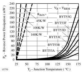
Figure 2. Max. Reverse Power Dissipation vs. Junction Temperature
