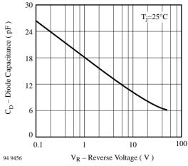
Figure 6. Typ. Diode Capacitance vs. Reverse Voltage
