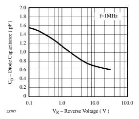
Figure 4. Diode Capacitance vs. Reverse Voltage
