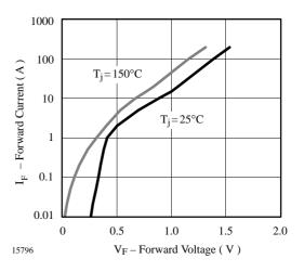
Figure 3. Forward Current vs. Forward Voltage
