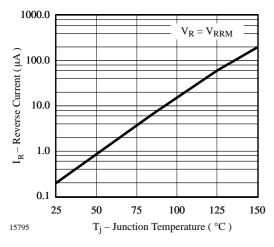
Figure 2. Reverse Current vs. Junction Temperature
