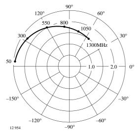
Figure 10. Forward transmission coefficient
