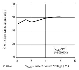
Figure 8. Cross Modulation vs. Gate 2 Source Voltage
