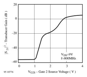
Figure 7. Transducer Gain vs. Gate 2 Source Voltage
