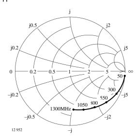
Figure 9. Input reflection coefficient
