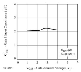
Figure 5. Gate 1 Input Capacitance vs. Gate 2 Source Voltage
