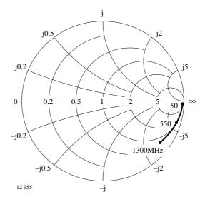
Figure 12. Output reflection coefficient
