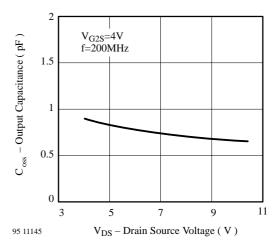
Figure 6. Output Capacitance vs. Drain Source Voltage
