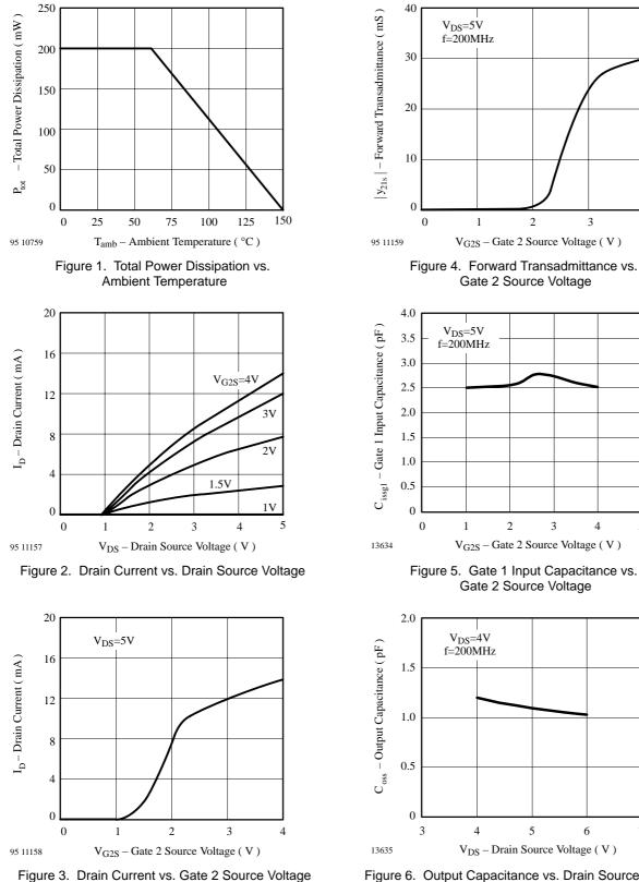
Figure 6. Output Capacitance vs. Drain Source Voltage
