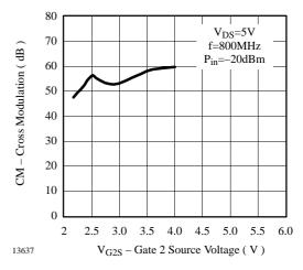
Figure 8. Cross Modulation vs. Gate 2 Source Voltage
