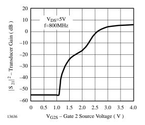
Figure 7. Transducer Gain vs. Gate 2 Source Voltage
