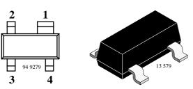
S595T Marking: 595 Plastic case (SOT 143) 1 = Source, 2 = Drain, 3 = Gate 2, 4 = Gate 1
