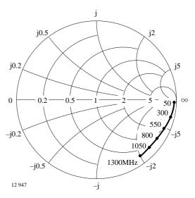
Figure 12. Output reflection coefficient
